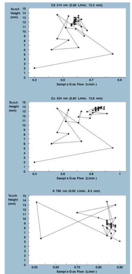
Actual auto-optimisation for 3 different elements. Note that the optimum torch viewing height and nebuliser flows are different.
