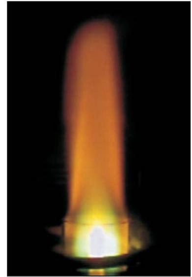
ICP users often look at the Plasma to determine quickly whether either the sample has reached the plasma or whether the rinse solution has flushed it out. With an optional Plasma Cam™, the end user can now view this and more from the convenience of the computer screen.
