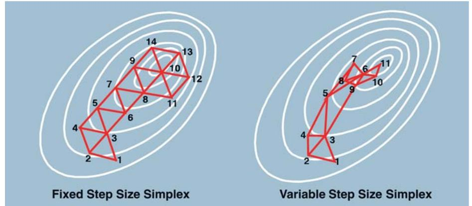
A variable step size simple algorithm allows faster, more precise and accurate optimisation compared to a fixed step
