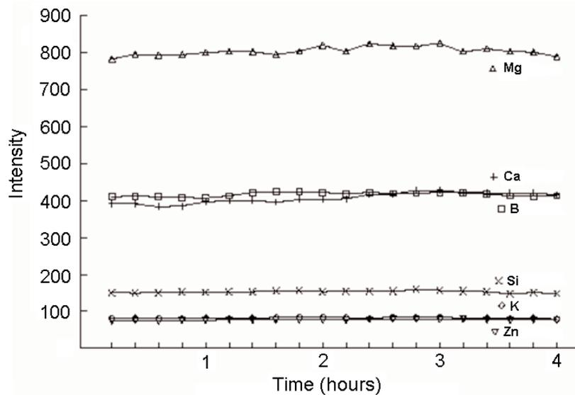
30% NaCl solution excellent reproducibility over 4 hours using standard sample introduction components and Argon Humidifier.
