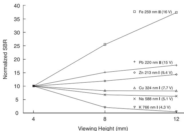
Graphs showing effect that varying viewing height and nebuliser flow have on various elements.
